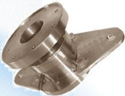
**Rotary joint**, provides a mechanical seal between a stationary supply pipe and a rotating drum or cylinder to permit the flow of heat transfer media, or just water into and/or out of the rotating element.
